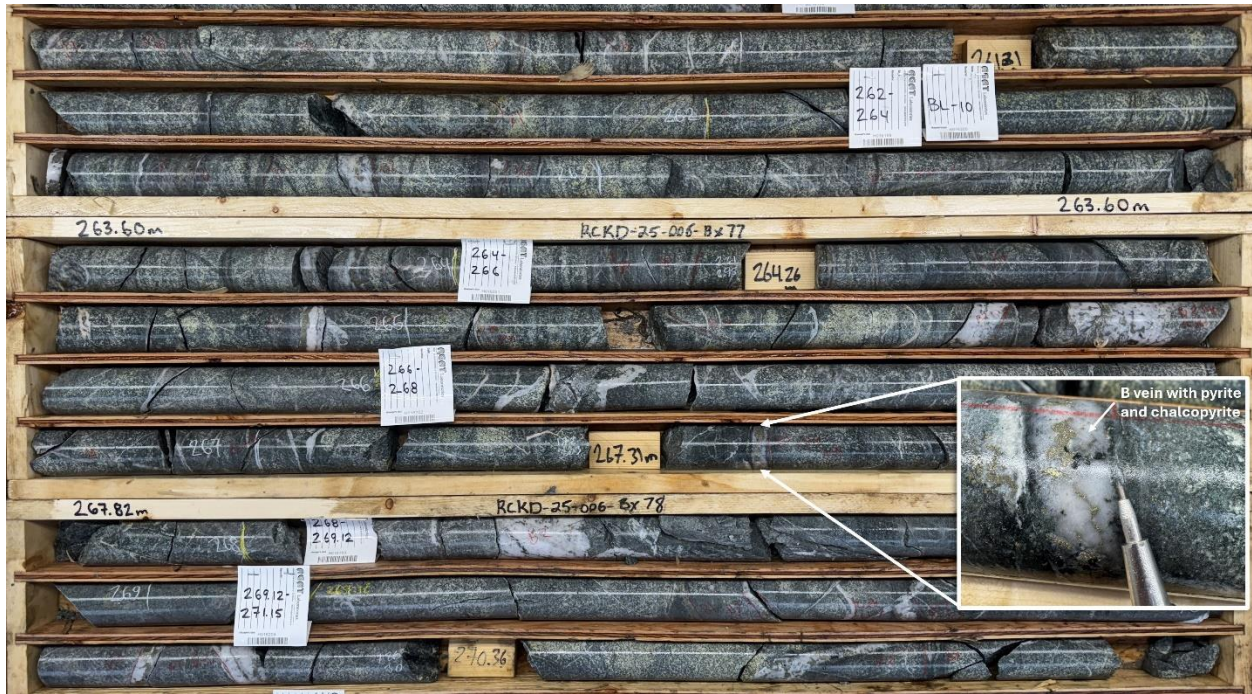
Figure 6: RCKD-25-006 NQ drill hole showing an altered porphyry intrusion and associated B-style veins.
