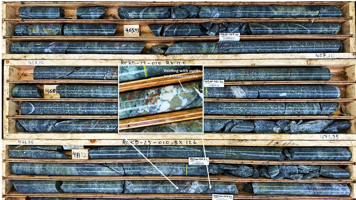
Figure 5: RCKD-25-010 NQ drill hole showing brecciated, altered porphyry intrusive and volcanic rocks with associated fracture filled veins and B-type veins.
